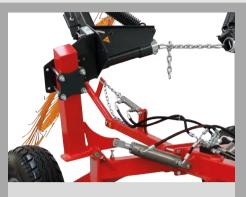
An hydraulically controlled mechanism converts the machine from transport to work position in only a few seconds. The working width and the angle of the finger wheels are easily adjustable to requirements based on the type and conditions of the harvest.
