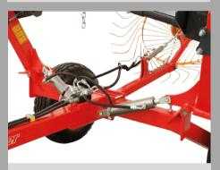
With the adjustable rake wheel downpressure spring. You can match the rake to your crop conditions. Use less downpressure for light hay or more downpressure for heavier hay. By minimizing down pressure, you extend the life of your rake tines and decrease the amount of debris collected in your window.
